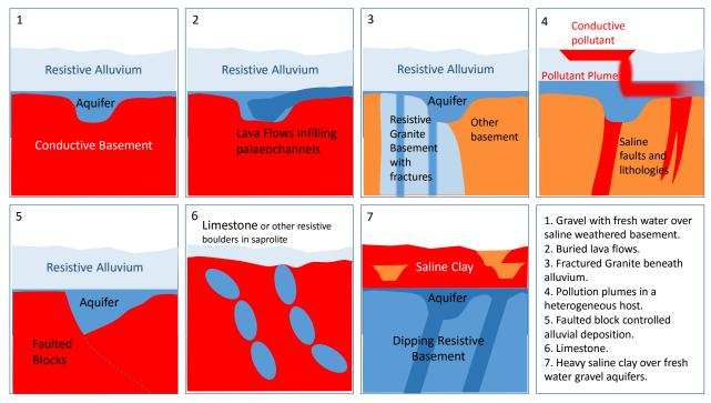
Figure 2 Conceptual models of typical TEM targets. Notice that in many cases the target is far from ideal in terms of resolvability using TEM yet, with sufficient consideration of survey design these problems can be resolved.
