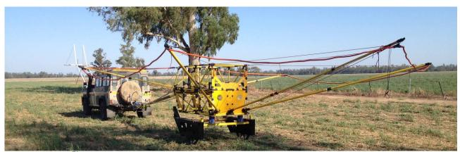
Figure 1: AgTEM4<sup>™</sup> cart with an additional receiver loop forward of the towing vehicle.
